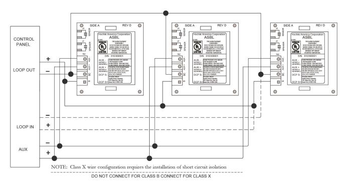
NOTE: Fire alarm control panel compatibility is required for DCP products. DCP communications protocol allows system components (DCP sensors AIE-EA, ALG-V, ACA-V, ACC-V, ALK-V, ALN-V, ATJ-EA, ATG-EA, ACD-V, bases and modules) to be used concurrently on a system's SLC (Signaling Line Circuit).
