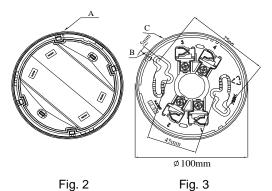
Connection: Loop of the control panel should be connected with terminals "1" and "3" of the base, polarized-insensitive; terminals "2" to anode of remote indicator and "4" to the cathode.
